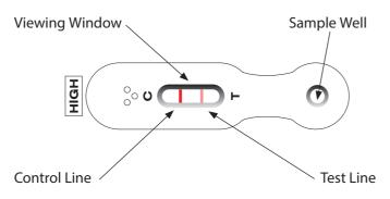
There is an in built Control in the test and for all samples run; a line should appear against the C (Control) point in the viewing window. If no line appears the test has failed and should be repeated.
