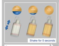
For all types of test, secure dropper cap and shake sample vigorously for 5 seconds
