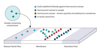
The gold-labelled antibody is immobilised in the Release Pad under the sample well. The sample containing an unknown amount of contamination is added to the sample well and this re-hydrates, allowing the reagents to flow up (wicking) the membrane towards the absorbent pad. Any large particles in the sample, which may
