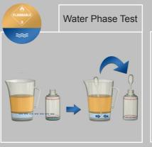
If enough water is free in the sample use the pipette to fill the bottle to lower line
