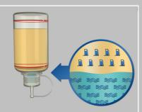
Invert bottle and allow blue fluid to settle out of the fuel sample.
