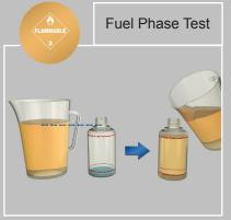
If no water is visible in the sample, fill the bottle to the top line with fuel
